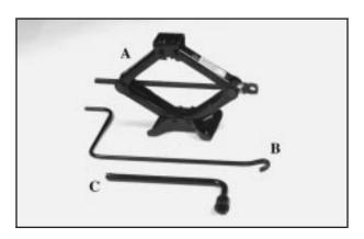
The tools you'll be using include the jack (A), jack handle (B) and wheel wrench (C).
